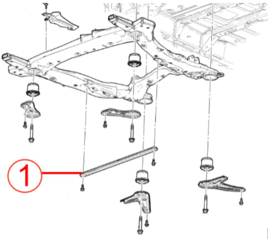
**Remove the cradle brace and drive the vehicle under the conditions that will duplicate the noise.**
