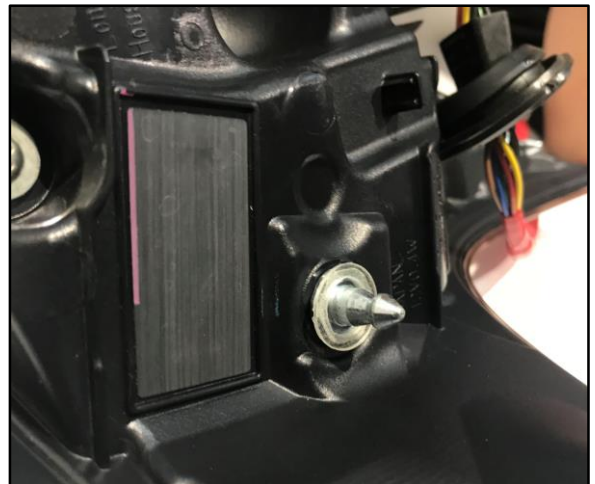
Figure 6. Washer Installed to Upper Guide Pin
