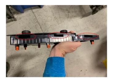
3 pieces of tape applied to top of IC stack
