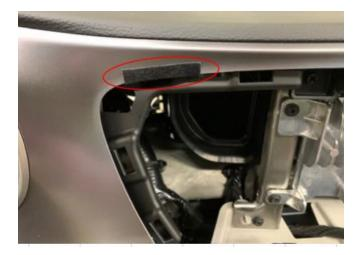
1 piece attached to upper left of Integrated Center Stack Bezel opening. **NOTE>>>** Tape should not be visible with the bezel installed.
