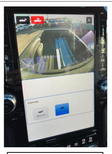
**Correct Operation:** CHMSL / Cargo Camera should not be blue and AUX should work if equipped
