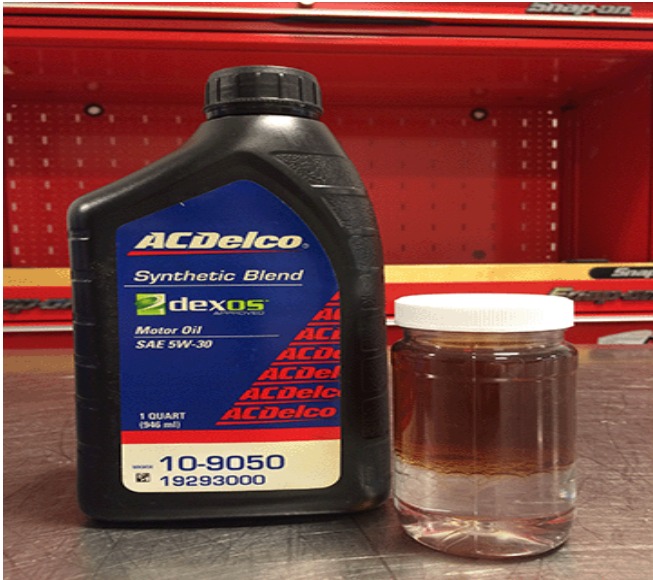
Diesel Exhaust Fluid (DEF) mixed with Diesel Fuel.
