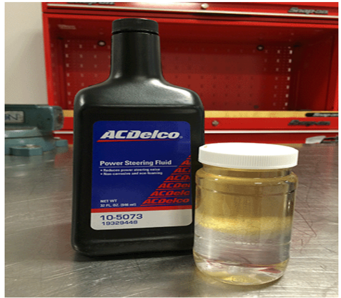
Diesel Exhaust Fluid (DEF) mixed with Power Steering Fluid.
