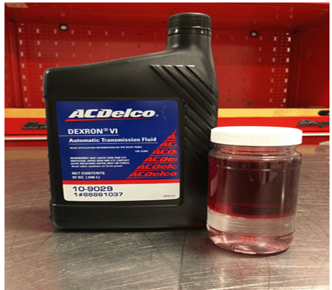
Diesel Exhaust Fluid (DEF) mixed with Power Steering Fluid.
