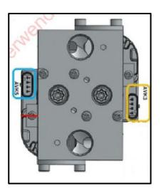
• Check air conditioner valve block wiring and replace harness, if necessary.
