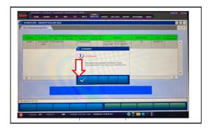
j. Verify the software by turning the ignition switch to the ON position and select the "Special Function" button under the HVAC tab.
