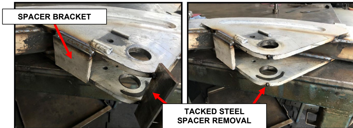
Figure 10 Weld Spacer Bracket and Remove Steel Spacer
