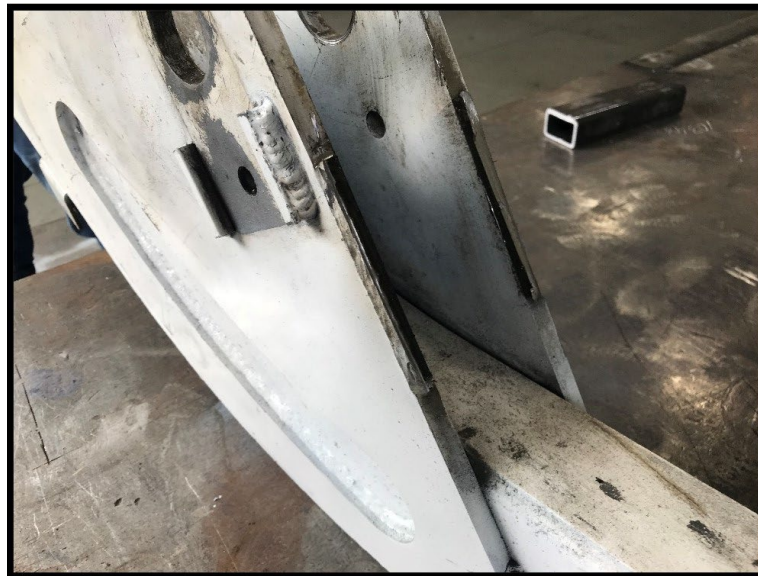
Figure 5 Removed Spacer Bracket
