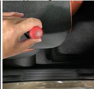
6. While holding the linkage upward (red arrow), insert the release button (yellow) into the seat belt guide assembly and press firmly until it engages the linkage.
