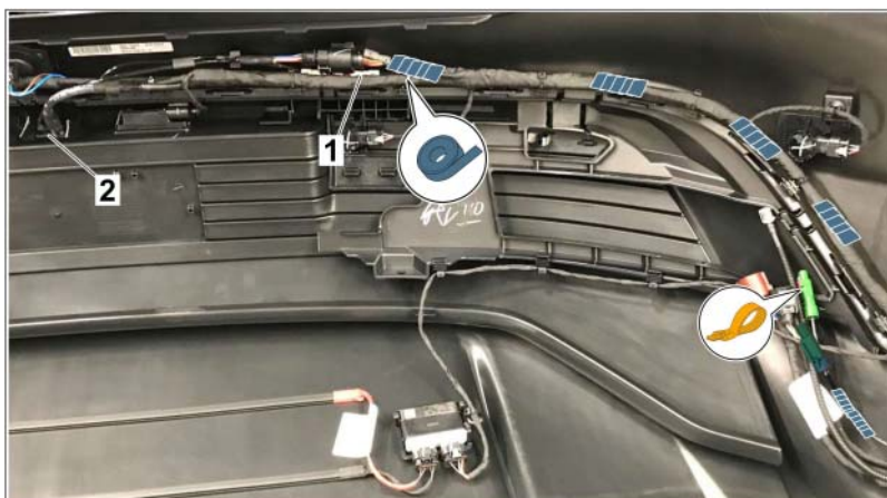
Connecting antenna cable for reversing camera
