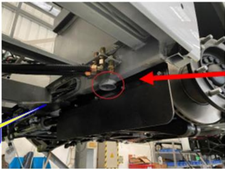
Front jack stand location, behind the front axle
