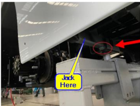
Front jack stand location, behind the front axle
