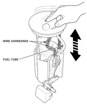
33. Install the new O-ring to the fuel tank, then partially install the new fuel tank unit and connect the transfer pipe quickconnect fitting.
