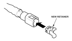
39. Connect the fuel line quick-connect fitting.
