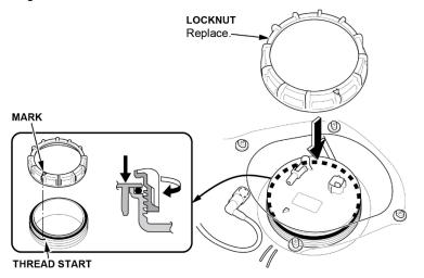
36. Press down on the fuel tank unit while turning the locknut clockwise by hand.
