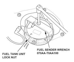
12. Remove the fuel tank unit.
