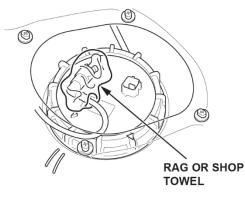
11. Remove the fuel tank unit locknut using the fuel sender wrench (T/N 070AA-T0AA100) as shown.
