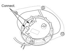
40. Connect the fuel tank unit connector.
