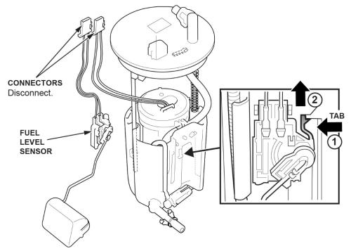
17. Disconnect the fuel level sensor harness and remove the fuel level sensor from the fuel tank unit.
