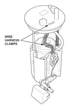
16. Press the tab on the fuel level sensor to release the lock. Then, push up on the fuel level sensor.
