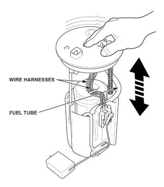
31. Install the new O-ring to the fuel tank, then partially install the new fuel tank unit.
