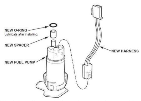
24. Install the new harness and make sure the connection is secure and the connectors are firmly locked into place.
