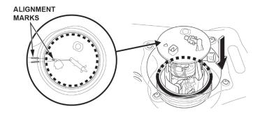
33. Line up the mark on the new locknut to the start of the thread on the fuel tank.
