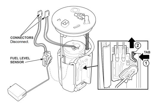
16. Disconnect the fuel level sensor harness and remove the fuel level sensor from the fuel tank unit.
