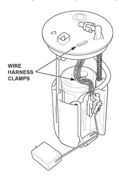
15. Press the tab on the fuel level sensor to release the lock. Then, push up on the fuel level sensor.
