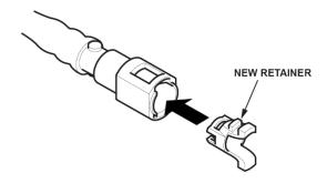
37. Connect the fuel line quick-connect fitting.
