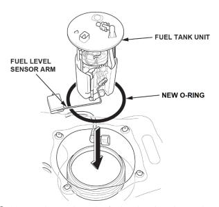
32. Line up the mark on the fuel tank unit to the marks on the fuel tank, then insert the fuel tank unit into the fuel tank. NOTE: To avoid any leaks, check the O-ring, either visually or by hand, to make sure it is not pinched.
