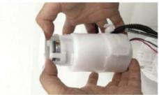
26. Install the fuel filter assembly to the reservoir.
