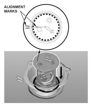
43. Line up the mark on the new locknut to the start of the thread on the fuel tank.
