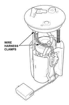
26. Press the tab on the fuel level sensor to release the lock. Then, push up on the fuel level sensor.
