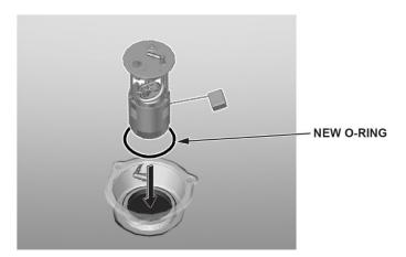
42. Line up the mark on the fuel tank unit to the marks on the fuel tank, then insert the fuel tank unit into the fuel tank. NOTE: To avoid any leaks, check the O-ring, either visually or by hand, to make sure it is not pinched.
