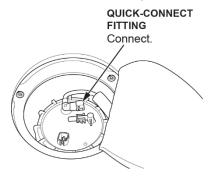
48. Connect the fuel tank unit connector.
