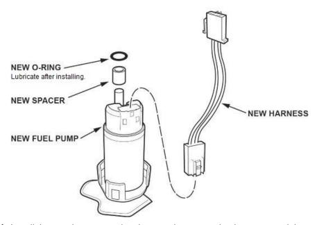
34. Install the new harness and make sure the connection is secure and the connectors are firmly locked into place.
