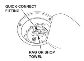
21. Disconnect the quick-connect fitting from the fuel tank unit.
