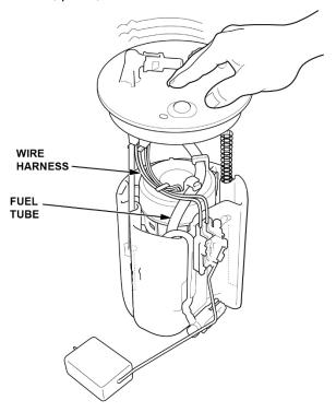
41. Insert the fuel tank unit partially into the fuel tank with a new O-ring.
