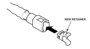
47. Connect the fuel line quick-connect fitting.
