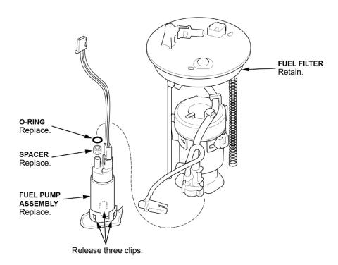
31. Pull the fuel pump assembly out of the fuel filter.
