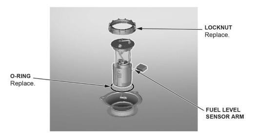
24. Prepare the fuel tank unit and parts to be replaced.
