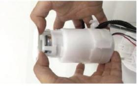
36. Install the fuel filter assembly to the reservoir.
