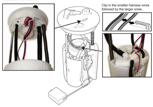
40. While compressing the fuel tank unit, make sure the movement is smooth and the fuel tube and wiring harness do not stretch, pinch, or bind.
