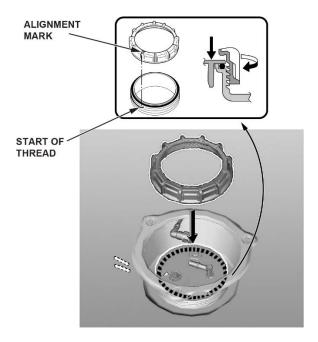
44. Press down on the fuel tank unit while turning the locknut clockwise by hand.
