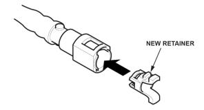
40. Connect the fuel line quick-connect fitting.
