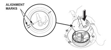
36. Line up the mark on the new locknut to the start of the thread on the fuel tank.
