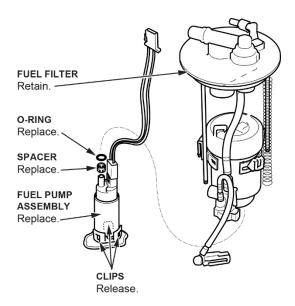
24. Pull the fuel pump assembly out of the fuel filter.
