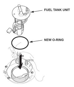
35. Line up the mark on the fuel tank unit to the marks on the fuel tank, then insert the fuel tank unit into the fuel tank. NOTE: To avoid any leaks, check the O-ring, either visually or by hand, to make sure it is not pinched.
