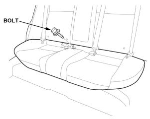
5. While pushing down on the rear seat cushion, pull the seat hook handles to release the hooks.
