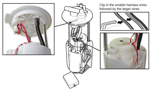
33. While compressing the fuel tank unit, make sure the movement is smooth and the fuel tube and wiring harness do not stretch, pinch, or bind.
