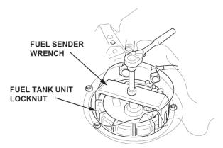
15. Remove the fuel tank unit.
