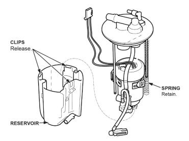
23. Release the three clips at the base of the fuel pump assembly and remove it from the fuel filter.
