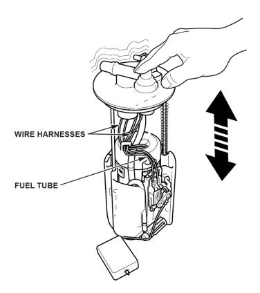
34. Install the new O-ring to the fuel tank, then partially install the new fuel tank unit.
