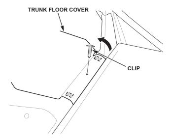
10. Open the trunklid, then remove the trunk floor cover.
