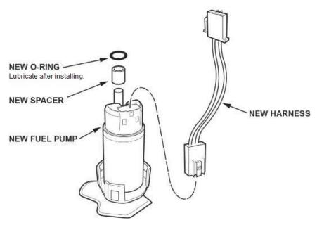
27. Install the new harness and make sure the connection is secure and the connectors are firmly locked into place.
