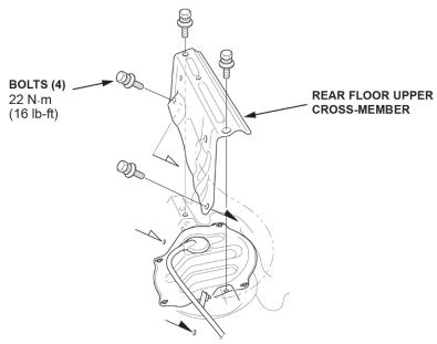
12. Remove the fuel tank unit access panel and disconnect the connector.
