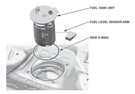
37. Line up the tab of the fuel tank unit as shown, and partially install the new fuel tank unit cam lock ring with a new O-ring.
