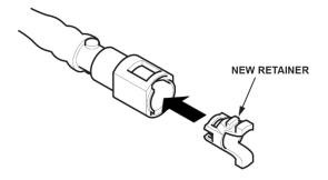
41. Connect the fuel line quick-connect fitting.
