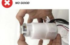
31. Install the fuel filter assembly to the reservoir.
