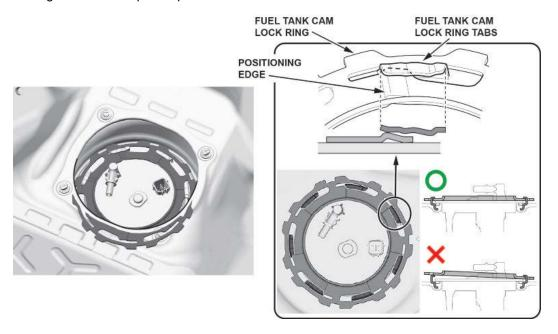
39. Tighten the fuel tank unit cam lock ring by turning clockwise using the fuel sender wrench.
