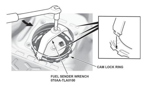
17. Turn the fuel tank unit cam lock ring counterclockwise to unlock it.
