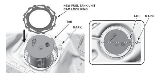
38. Turn the fuel tank unit cam lock ring by hand, and slide the fuel tank unit cam lock tabs to the positioning edge as shown.
