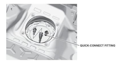
42. Connect the fuel tank unit connector.
