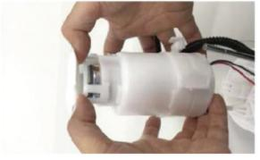
33. Install the fuel filter assembly to the reservoir.
