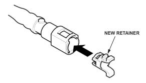
43. Connect the fuel line quick-connect fitting.
