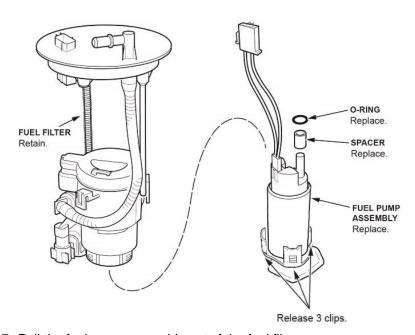
27. Pull the fuel pump assembly out of the fuel filter.
