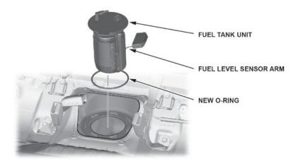
38. Line up the tab of the fuel tank unit as shown, and partially install the new fuel tank unit cam lock ring.
