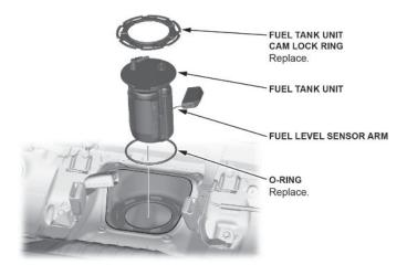
20. Prepare the fuel pump and parts to be replaced.
