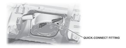
44. Connect the fuel tank unit connector.
