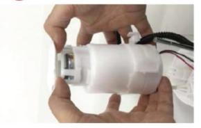
32. Install the fuel filter assembly to the reservoir.
