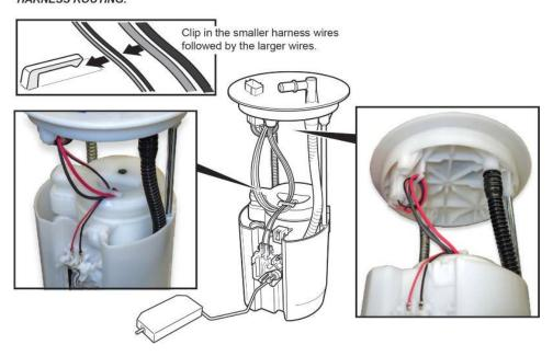
36. While compressing the fuel tank unit, make sure the movement is smooth and the fuel tube and wiring harness do not stretch, pinch, or bind.
