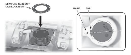
39. Tighten the fuel tank unit cam lock ring.
