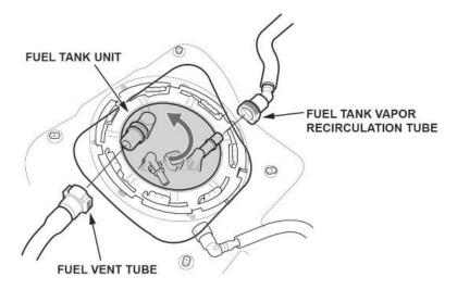
58. Turn the fuel tank unit cam lock ring by hand, and slide the fuel tank unit cam lock tabs to the positioning edge as shown.
