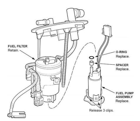
42. Install the new spacer on the new fuel pump motor.
