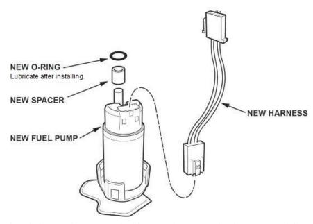
44. Install the new harness and make sure the connection is secure and the connectors are firmly locked into place.
