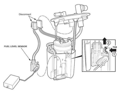
38. Disconnect the fuel level sensor harness and remove the fuel level sensor from the fuel tank unit.
