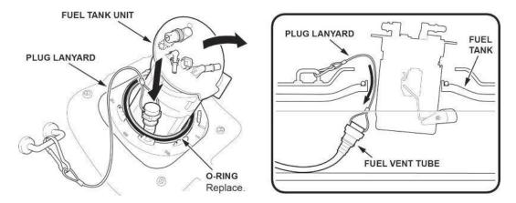
34. Remove the fuel tank unit with the O-ring.
