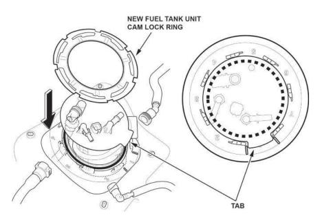
58. Connect the fuel vent tube and fuel tank vapor recirculation tube by slightly turning the fuel tank unit counterclockwise. NOTE: Do not bend the fuel vent tube and fuel tank vapor recirculation tube excessively.
