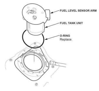
35. Prepare the fuel tank unit and parts to be replaced.
