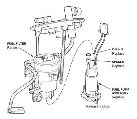
43. Install the new spacer on the new fuel pump motor.
