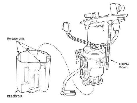
42. Release the three clips at the base of the fuel pump assembly and remove it from the fuel filter.
