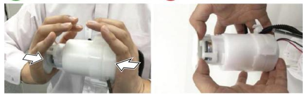
47. Install the fuel filter assembly to the reservoir.
