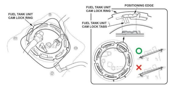
60. Tighten the fuel tank unit cam lock ring by turning clockwise using the fuel sender wrench.
