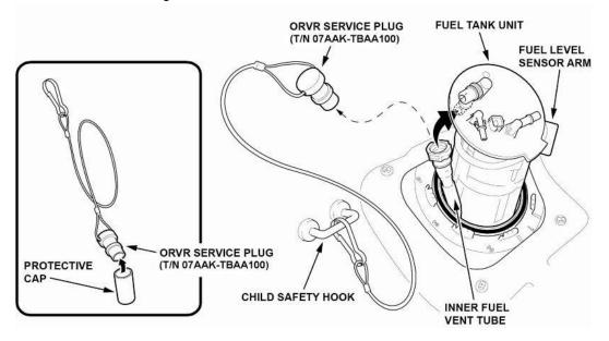
56. Remove the ORVR service plug from the child safety seat hook, and install the provided protective cap.
