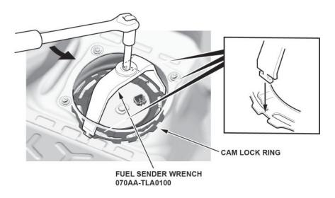
18. Turn the fuel tank unit cam lock ring counterclockwise to unlock it.
