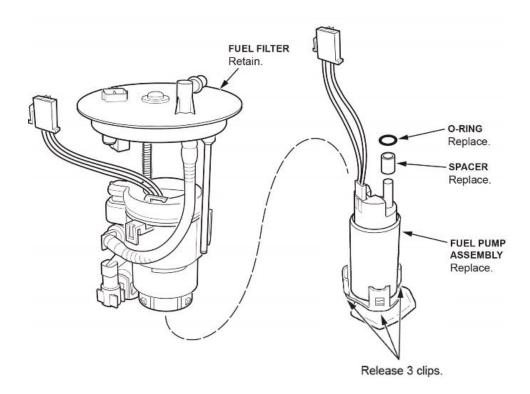
27. Pull the fuel pump assembly out of the fuel filter.
