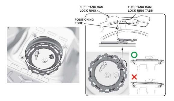
39. Tighten the fuel tank unit cam lock ring by turning it clockwise using the fuel sender wrench.
