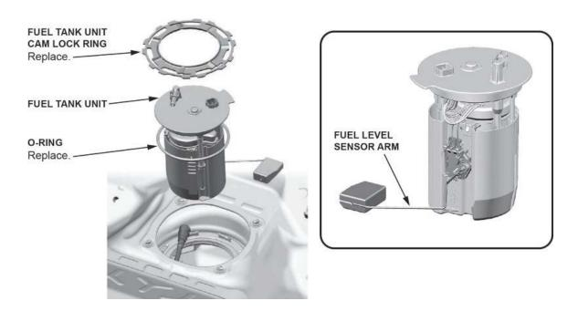
20. Prepare the fuel pump and parts to be replaced.
