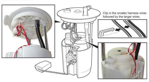
36. While compressing the fuel tank unit, make sure the movement is smooth and the fuel tube and wiring harness do not stretch, pinch, or bind.
