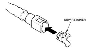
41. Connect the fuel line quick-connect fitting.
