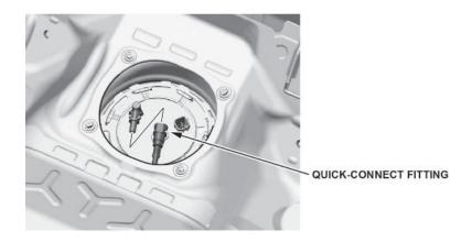
42. Connect the fuel tank unit connector.
