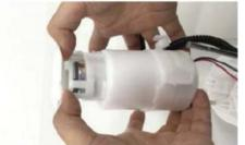
31. Install the fuel filter assembly to the reservoir.
