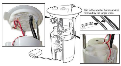
35. While compressing the fuel tank unit, make sure the movement is smooth and the fuel tube and wiring harness do not stretch, pinch, or bind.
