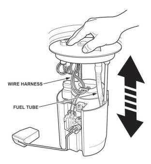
36. Install the fuel tank unit into the fuel tank with a new O-ring.
