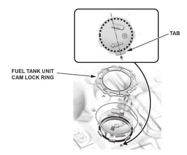
48. Rotate the fuel tank unit cam lock ring and slide the fuel tank unit cam lock tabs into the positioning edge slightly as shown by hand.
