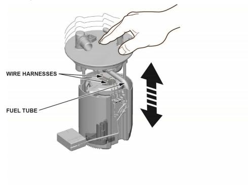
42. Install the fuel tank unit into the fuel tank with a new O-ring.
