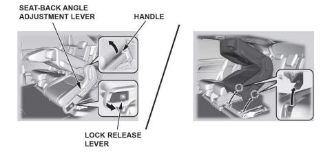
Pull the lock release lever, tilt the seat-back forward and the lift the rear of the seat.
