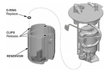
31. Release the three clips at the base of the fuel pump assembly and remove it from the fuel filter.
