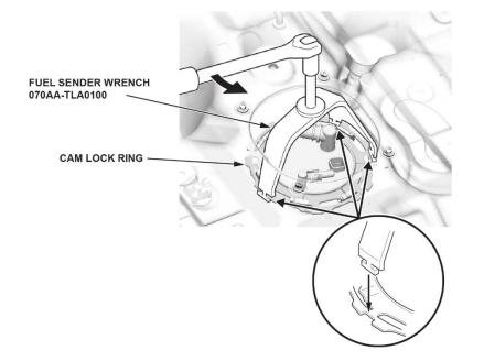
18. Turn the fuel tank unit cam lock ring counterclockwise to unlock it.
