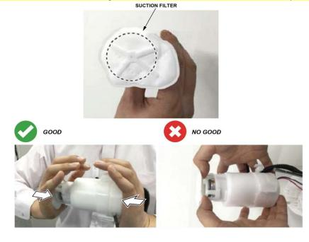
37. Install the fuel filter assembly to the reservoir.
