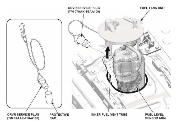
46. Remove the ORVR service plug from the child safety seat hook, and install the provided protective cap.
