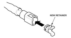
51. Connect the fuel vapor hose, the fuel line quick-connect fitting, and fuel tank unit connector.
