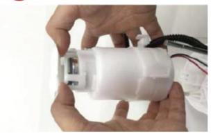
30. Install the fuel filter assembly to the reservoir.
