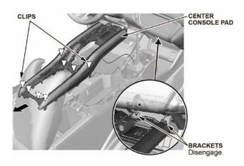
15. Remove the center console rear trim, and disconnect the connector.
