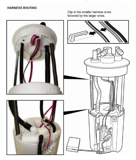
44. While compressing the fuel tank unit, make sure the movement is smooth and the fuel tube and wiring harness do not stretch, pinch, or bind.
