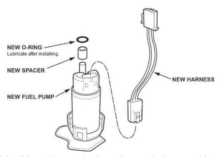
38. Install the new harness and make sure the connection is secure and the connectors are firmly locked into place.
