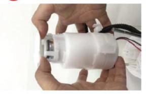
40. Install the fuel filter assembly to the reservoir.
