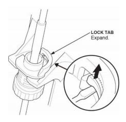
• Rotate the socket holder retainer counterclockwise until it stops, then remove the shift cable. NOTE: Do not remove the shift cable by pulling the shift cable guide.
