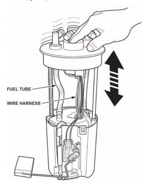
45. Partially insert the fuel tank unit into the fuel tank with a new base gasket.
