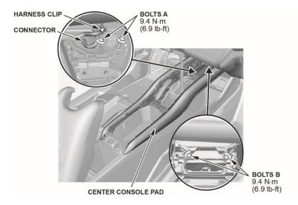
14. Remove the center console pad, and disengage the brackets from the bolts.
