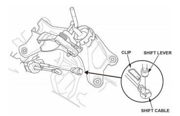
• Disconnect the shift cable from the shift lever.
