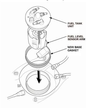
46. Line up the marks on the fuel tank and fuel tank unit as shown, then insert the fuel tank unit.
