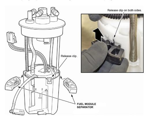
34. Release the three clips at the base of the fuel pump assembly.
