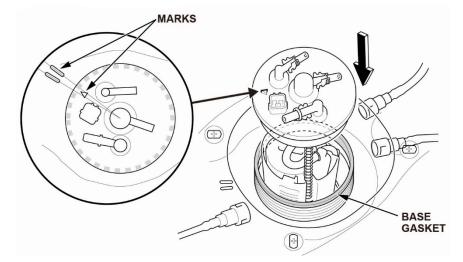
22. Tighten the fuel tank unit locknut.
