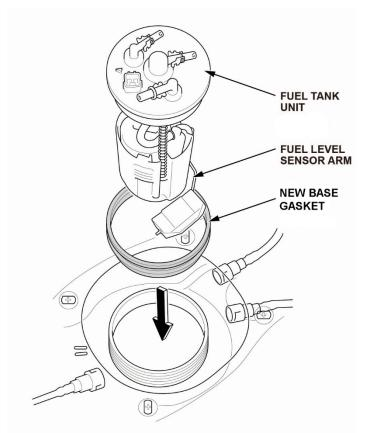
21.2. Line up the marks on the fuel tank and fuel tank unit as shown, then insert the fuel tank unit.
