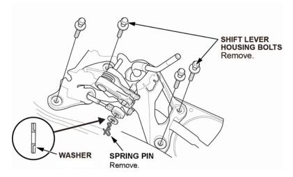
13.2 Remove the shift lever housing bolts.
