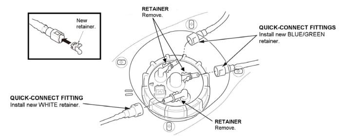
24. Connect the quick-connect fittings to the fuel tank unit.
