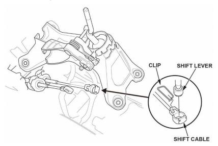
13.7 Disconnect the shift cable from the shift lever.
