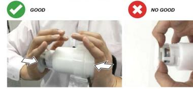
20.5. Install the fuel filter assembly to the reservoir.
