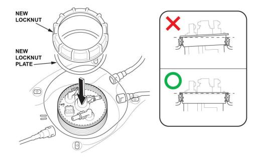
15.2. Tighten the fuel tank unit locknut to the specified torque using the fuel sender wrench.
