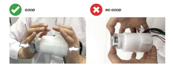
13.5. Install the fuel filter assembly to the reservoir.
