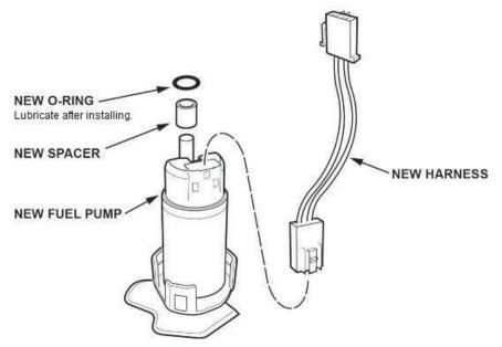
13.3. Install the new harness and make sure the connection is secure and the connectors are firmly locked into place.
