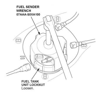
11. Remove the fuel tank unit locknut, then remove the fuel tank unit.
