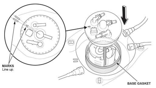
15. Tighten the fuel tank unit locknut.
