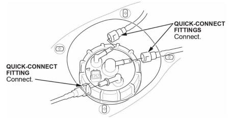
18. Connect the fuel tank unit connector.
