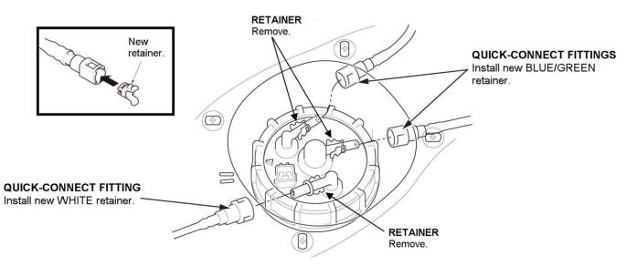
17. Connect the quick-connect fittings to the fuel tank unit.
