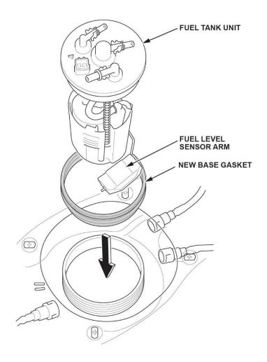
14.2. Line up the marks on the fuel tank and fuel tank unit as shown, then partially install the fuel tank unit. NOTE: To avoid a fuel leak, visually or by hand, make sure the base gasket is not pinched.
