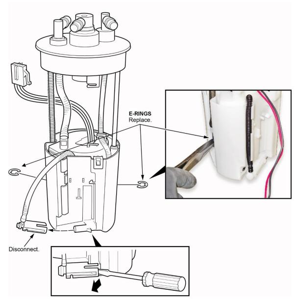
12.5. Disconnect the joint at the bottom of the reservoir.
