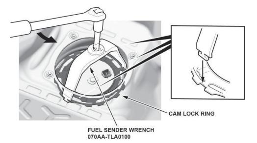
6.2. Turn the fuel tank unit cam lock ring counterclockwise.
