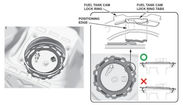
11.2. Turn the fuel tank unit cam lock ring clockwise using the fuel sender wrench.
