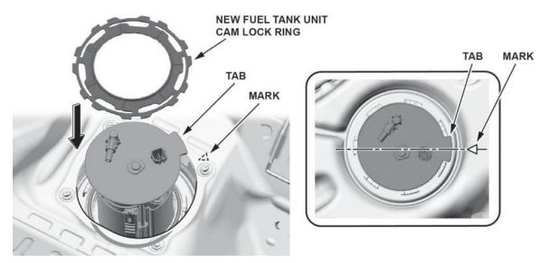
11. Lock the fuel tank unit cam lock ring.
