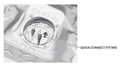
14. Connect the fuel tank unit connector.
