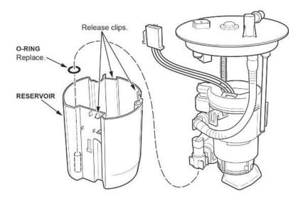
8.6. Remove the fuel pump assembly from the fuel filter.
