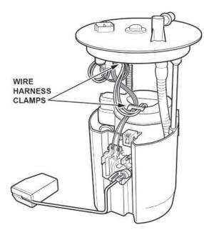
8.3. Remove the fuel level sensor.
