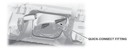
15. Connect the fuel tank unit connector.
