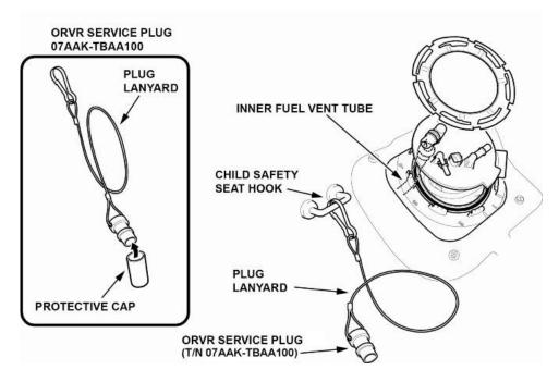
12.2. Disconnect the inner fuel vent tube from the fuel tank unit, and hold it. Do not allow the inner fuel vent tube to drop into the fuel tank.
