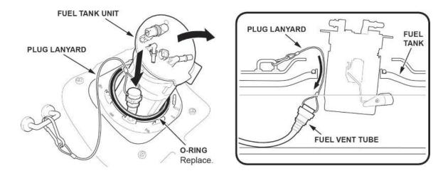
12.5. Remove the fuel tank unit with the O-ring.
