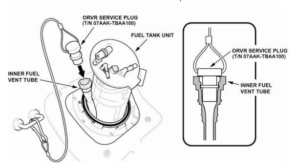
12.3. Install the ORVR service plug to the inner fuel vent tube. Make sure the ORVR service plug is fully seated by holding the inner fuel vent tube, and gently pulling on the plug's lanyard.
