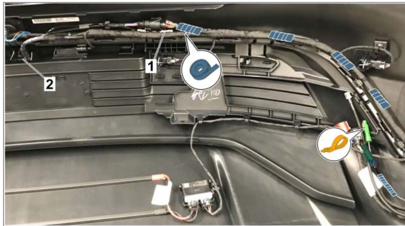
Connecting antenna cable for reversing camera
