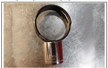
3. Preset the FRONT and BOTTOM clamps open on the fittings as shown.
