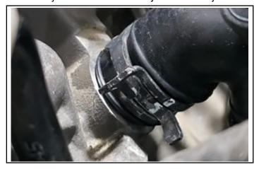
· Verify the REAR of coolant junction is fully seated.
