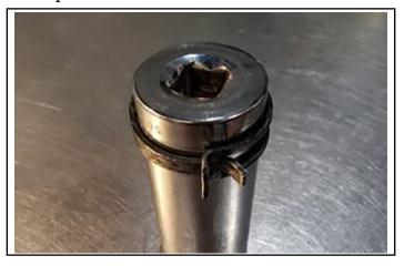
2. Install 13mm sockets over the FRONT and BOTTOM clamps to keep them in the open position.
