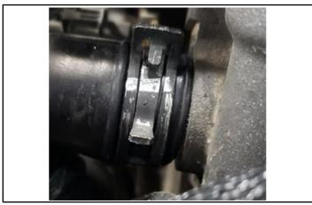
Verify the BOTTOM of coolant junction is fully seated.
