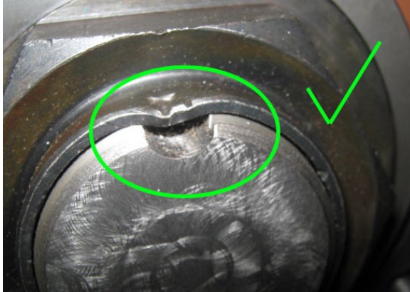
FIGURE 8: CORRECT - PREVENTS THE NUT FROM GETTING LOOSE
