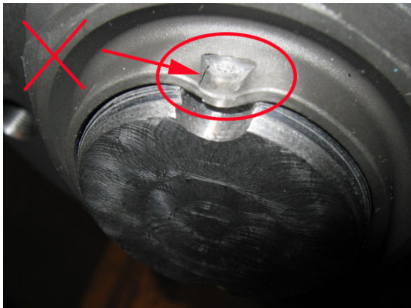
FIGURE 10: BROKEN OR TORN LIP – REJECTED
