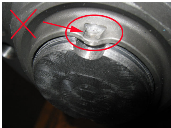
FIGURE 10: BROKEN OR TORN LIP – REJECTED
