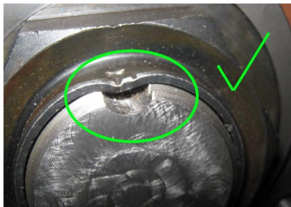
FIGURE 8: CORRECT - PREVENTS THE NUT FROM GETTING LOOSE
