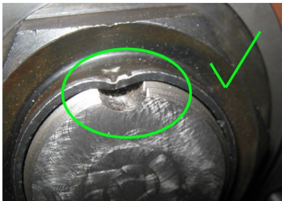
FIGURE 12: CORRECT - PREVENTS THE NUT FROM GETTING LOOSE
