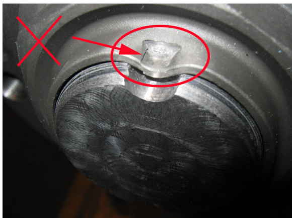
FIGURE 14: BROKEN OR TORN LIP – REJECTED
