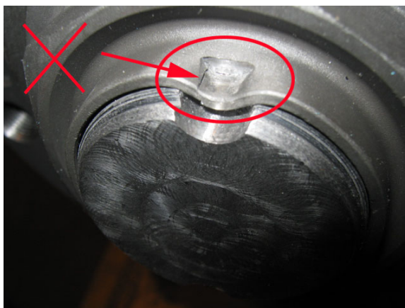
FIGURE 39: BROKEN OR TORN LIP – REJECTED
