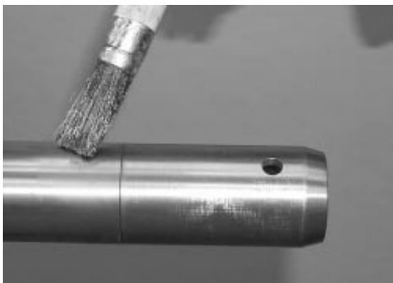
FIGURE 32: APPLY GLEITMO 805 GREASE
