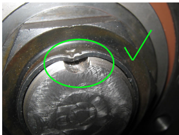
FIGURE 36: CORRECT - PREVENTS THE NUT FROM GETTING LOOSE
