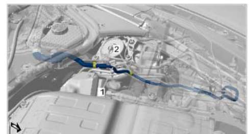
Securing return line in engine compartment
