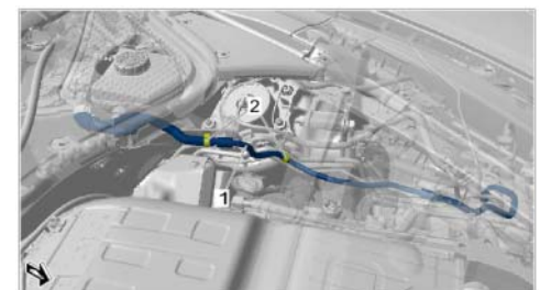
Loosen return line in the engine compartment.
