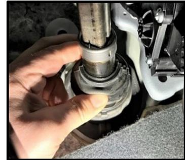
**STEP 2:** Push the dust seal in a downward direction away from the steering wheel. This will allow the old grease to be exposed.
