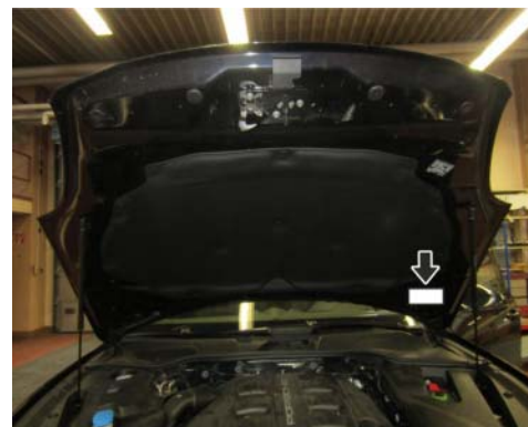
Proof of Completion Label: specified position (Exemplary illustration — Macan (95B) position accordingly)
