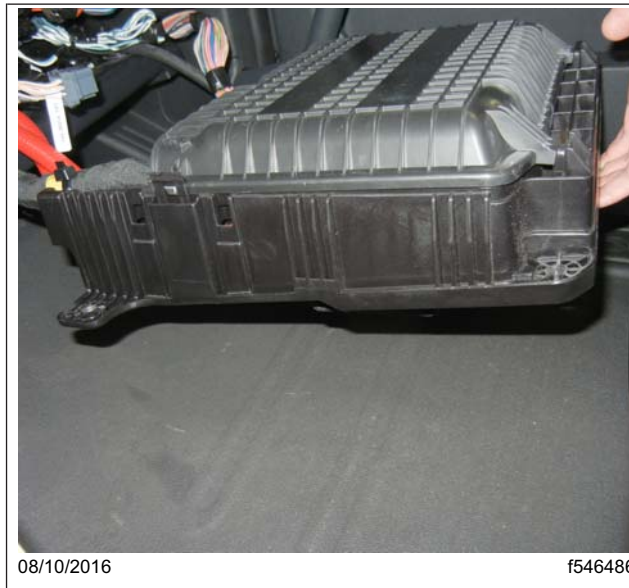
Fig. 10, Lowering the VPDM to the Cab Floor
