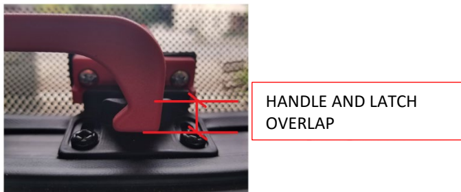
FIGURE 5 CORRECT HANDLE AND LATCH OVERLAP
