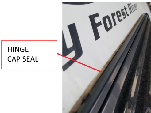
FIGURE 8 HINGE CAP SEAL
