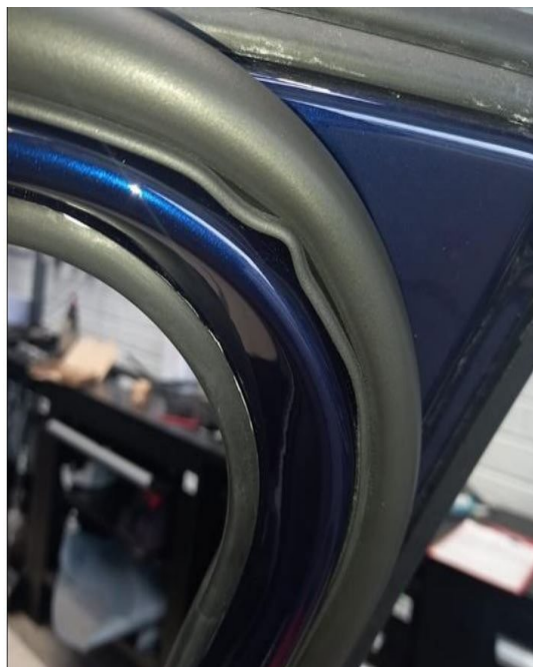
Figure 1. The outer door seal detached from the door.
