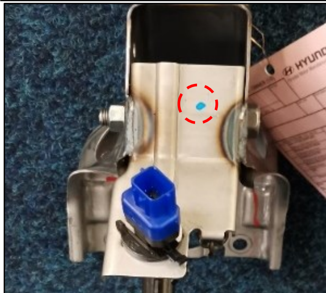
Blue dot – replacement necessary
