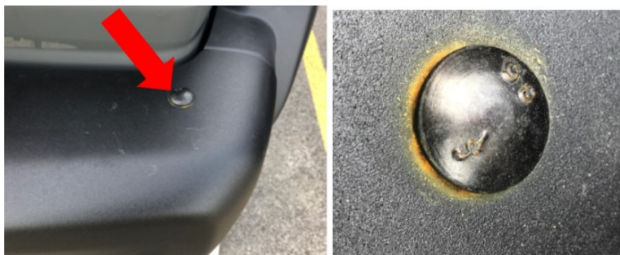
Fig. 1 Bumper Bolt Rust
