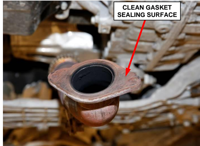
Figure 21 – Crossunder Pipe Flange
