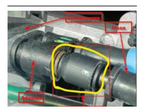
Intake/Exhaust hose assembly quick connect adaptor fitting
