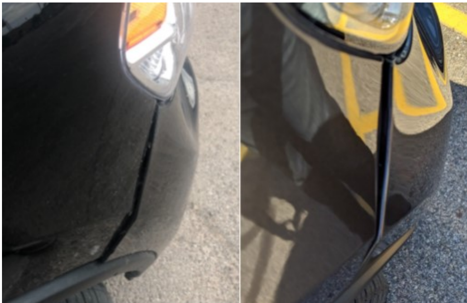
Fig. 1 Fender to Fascia Mis-Aligned
