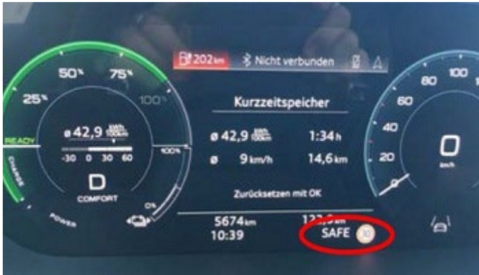
Figure 1: "SAFE" warning is shown by the instrument cluster
