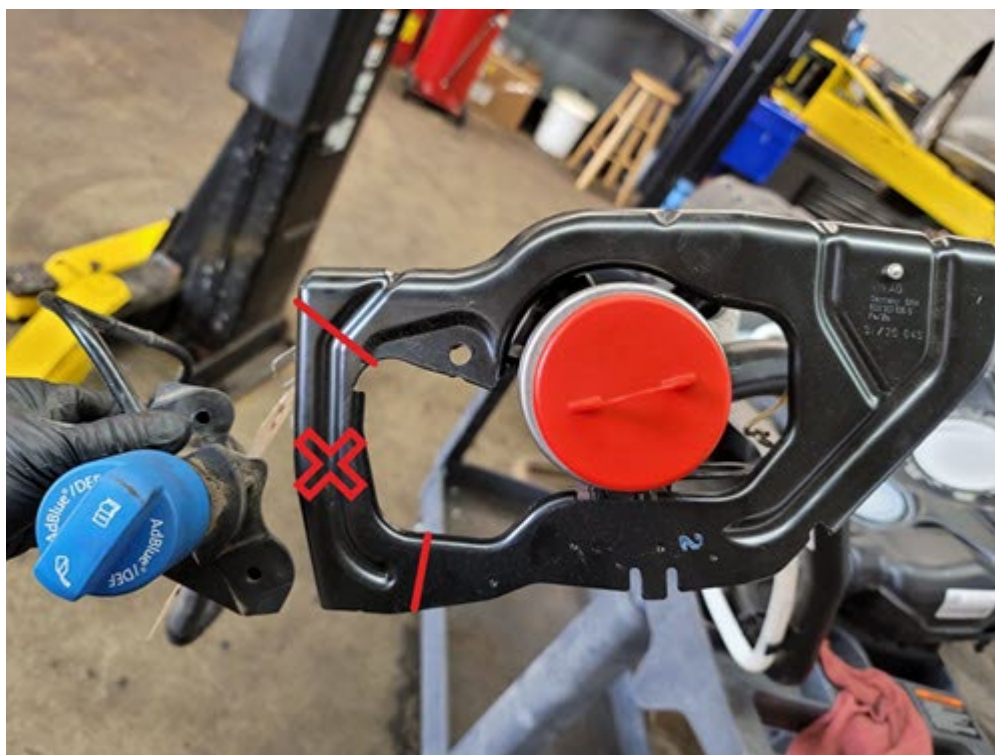
Figure 1: Remove the material indicated by the red X between the two red lines.
