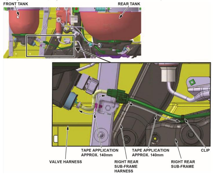
After repairing or replacing the harness, wrap some of that tape around the affected area. It has **capsaicin**. This should keep any critters from causing future problems.
