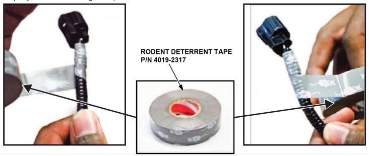
When wrapping the harness, use the method we refer to as half-wrapping. Each time you wrap the tape around the harness, overlap the layer you just did by half the width of the tape.
