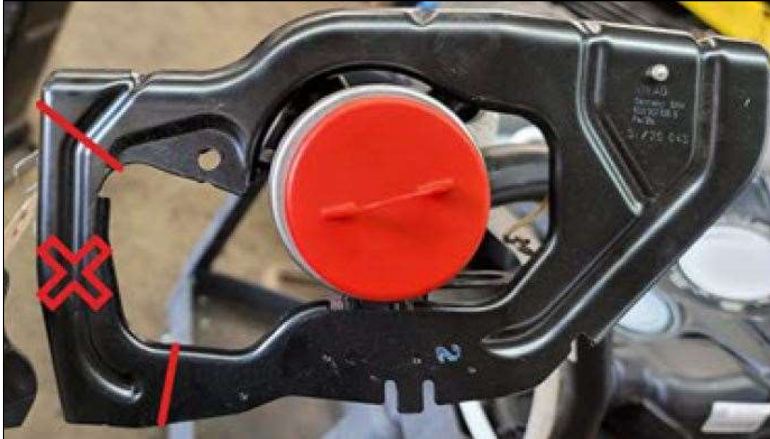
Figure 1: Remove the material indicated by the red X between the two red lines.
